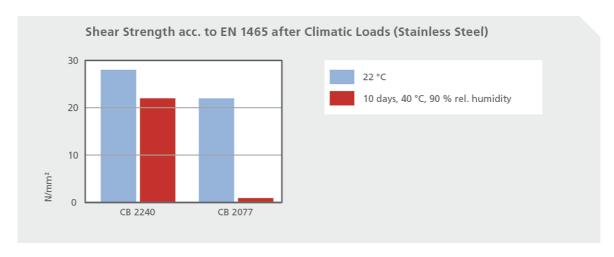
After a climatic load (10 days, 40°C, relative humidity 90%) **CB 2240** shows a shear value of around 22 N/mm2 and conclusively this strength was neither heavily influenced by adhesion or cohesion failure. This is different with standard products. After the climatic tests these standard adhesives did not show sufficient strength anymore.
