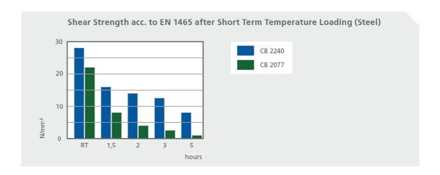
Another benefit of using Cyberbond xtraflex adhesives in industry is the gain in temperature resistance of these modified, partly flexible products. The short-term heat resistance in terms of shear strengths is increased substantially. These products show better results in all temperature ranges.
