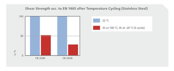
The diagram shows a lower decrease of strength after 5 cycles at 100 °C but at -20 °C for 3 hours the partly flexible Cyanoacrylate **CB 2240** retains much more of its initial strength, approx 52 percent, whereas the standard ethyl ester based Cyanoacrylate (**CB 2028**) only retains 28 percent.
