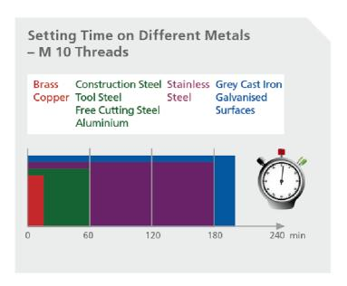
Curing time in minutes of an M 10 thread
