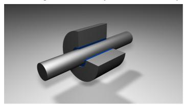
For inserted joints the size of the bonded surface is in relation to torque transfer. The surface relation (I/d) is defined as the ratio of the overlapping length (I) and diameter (d). An optimum tension per mm<sup>2</sup> is achievable with a surface relation of between I/d = 0.8 - 1.2. Smaller relations lead to tension peaks. By increasing the length over the optimum range the torque can be
