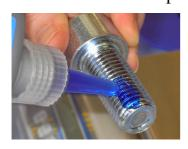
Vibration may cause problems such as the self-loosening of threads. By applying the Cyberbond "T" series grades, this problem is solved. Cyberbond maintains the on-torque given on a thread, which prevents the self-loosening process. At the same time Cyberbond fills the voids in the threads, which seals them and prevents corrosion. Liquid Cyberbond is simply applied straight from the bottle or tube. After assembly the product will cure completely and fix the mating parts. The complete thread
