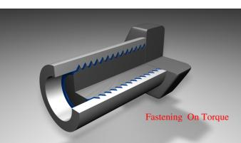
When dismantling and the break loose torque reached, the prevailing torque is of certain importance. This is the value you measure after the adhesive film has been broken. Dependent on the different chemicals within the adhesive the prevailing torque value can be higher or lower than the break loose torque. Once the adhesive film is broken there is no defined security left, no matter how high the prevailing torque finally is.
