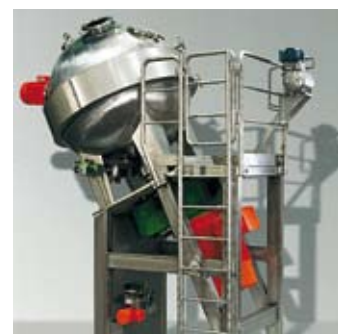
Spherical dryer (Rosenmund Guedu) for manufacturing pharmaceutical powders with HSMR5L-D.
