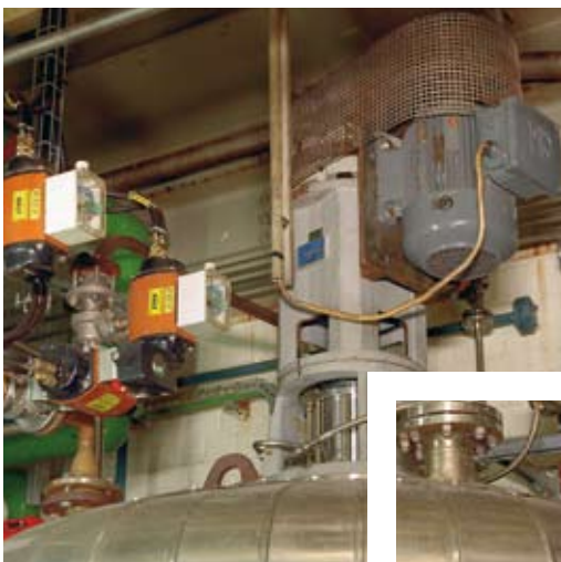
Polymers production at BASF Ludwigshafen. Stainless steel tank with top entry agitator.
