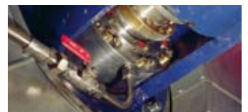
HSMR in a vacuum dryer
