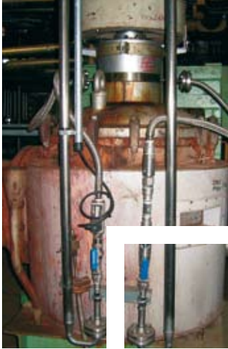
Thin-film evaporator (Chema) in the caprolactam plant at DOMO Capro Leuna.
