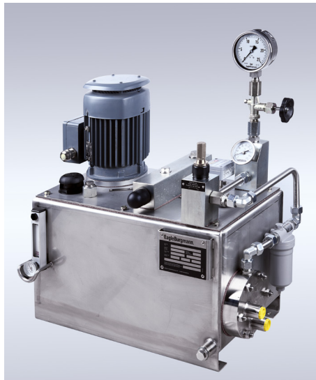
EagleBurgmann barrier system SPA 2000. Pressurized barrier fluid system type SPA in its basic version provide all four functions of a supply system which are necessary for the operation of double mechanical seals: barrier fluid circulation, cooling, pressure build-up in the sealing chamber and leakage compensation.
