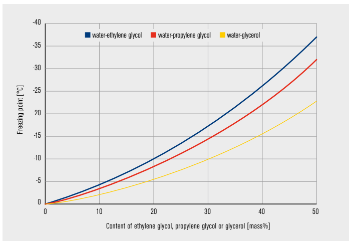
Freezing points of water-ethylene glycol, water-propylene glycol and water-glycerol mixtures Source: Internet, pro Kühleisole GmbH
