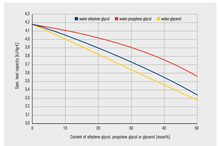
Specific heat capacity of water-ethylene glycol, water-propylene glycol and water-glycerol mixtures Source: Internet, pro Kühleisole GmbH
