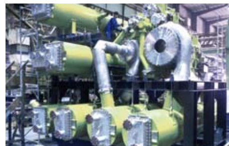
Multi-stage gear compressor Photo: MAN Diesel & Turbo SE
