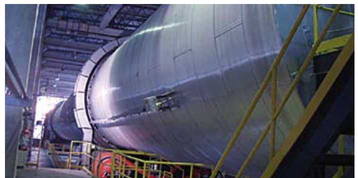
PET reactor Photo: M&G Polimeros Brasil S.A
