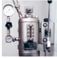
Thermosiphon system for supplying mechanical seals
