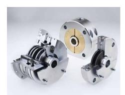
Carbon floating ring seals are supplied as maintenance free compact labyrinth cartridge seals with low leakage. The floating self-adjusting sealing rings provide radial sealing on the shaft with a very small gap. The seal requires no additional lubrication, and it is designed for dry running. Besides pure gas, carbon floating ring seals are also suitable for Atex applications, toxic media, media containing solids, flue gas, dust, powder, vapor, liquid mist, oil mist and penetrating oil.
