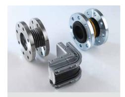
Flexible expansion joints in pipes and duct systems neutralize the effects of pressure and temperature fluctuation, vibration and misalignment at the joint. They must also be leakproof and resistant to media. Customized expansion joints made of fabric, metal or rubber are the solution of choice.
