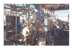
A **DGS11.1** seals a compressor in the fertilizer manufacturing facility at Incitec Pivot Limited in Australia. **Espey WD400** nitrogen-buffered carbon floating ring seals are used to seal the bearings. The process medium is a mixture of hydrogen and nitrogen. The seal is designed for frequent slow roll operation when starting and stopping the machine.
