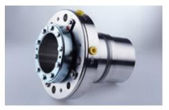
During the production of ammonia, carbon dioxide is removed from the process with Benfield solution – an aqueous potassium carbonate solution with diethanolamine. **HJS1** type mechanical seals have proven to be best for sealing the pumps in this area. Typical operating conditions:  $p=2\dots 4$  bar  $(29\dots 58\ PSI)$ ;  $t=100\dots 150\ ^{\circ}C\ (212\dots 302\ ^{\circ}F)$ ;  $n=1,500\ min^{-1}$ .
