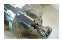
Bayer in Leverkusen, Germany, uses several screw spindle pumps to manufacture preproducts for polyurethane production that are sealed with **MAK66S3** type magnetic couplings. The process media are various polyethers with viscosities up to 3,500 mPas. Operating conditions: p=6 bar (87 PSI);  $t=20 \dots 80$  °C (68 ... 176 °F);  $n=350 \dots 1,500$  min<sup>-1</sup>.
