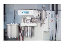
A Korean chemical company seals its Bühler bead mills for paint production with **MR1S1F-D24** type mechanical seals. The process medium – colored pigments with various solvents – is very abrasive.
