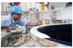
Tytan Organics Chemical Co. in the United Arab Emirates uses glass-lined reactor vessels to manufacture concrete plasticizers. The flanges and covers are sealed with **Burachem multi-gaskets** made from pure PTFE. Medium: Napthalene sulphonate formaldehyde. Operating conditions: p=6 bar (87 PSI); t=220 °C (428 °F).
