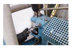
Liquid, high-purity ethylene is pumped in the cracker operated by the Dow Olefinverbund in Böhlen, Germany. The pump shaft is sealed by a **MFLCT80S1** type triple seal. The metal bellows seal has clear benefits at the temperatures down to  $-100~^{\circ}\text{C}~(-148~^{\circ}\text{F})$  encountered in this environment. A **TS2000** type Thermosiphon system supplies the seal.
