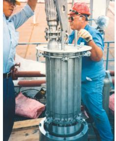
The high-efficiency **NMB-16P-2R-45-SC** magnetic coupling as a hermetic seal in a vertical pump. The process medium – a mixture of ammonia and propane – has very poor lubricating properties. The low temperature (–45 °C (–49 °F)) plays a decisive role in the choice of materials.
