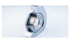
Gas-lubricated **MFLC-GS** metal bellows seals as single or double seals for the shafts of process pumps in air separation plants. Typical process media are liquefied gases such as nitrogen. The low temperatures require special materials for the secondary seals, such as the proven **Statotherm** graphite seals. Operating conditions: p = ... 25 bar (363 PSI); t = ... -199 °C (-326 °F); n = 6,000 ... 8,000 min<sup>-1</sup>.
