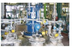
Sealing of polymerization reactors with an **HSMR5L-D** in the manufacture of synthetic rubber at Lanxess Deutschland GmbH. The process medium – monomers, water and polymers – has a tendency to bond. So flushing is used to protect the seal. An **SPA4025** buffer pressure system is used as the supply system.
