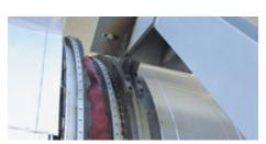
**DRO** Rotary kiln sealing system in a plant for incinerating chemical residues at Infracor GmbH at the Chemiepark in Marl, Germany.
