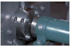
In a cracking unit in the United States a compressor is sealed by EagleBurgmann Espey carbon floating ring seals type **WD200** and **WDKS**. Operating conditions: p = ... 5 bar (73 PSI); t = 75 °C (167 °F); n = 3,000 min<sup>-1</sup>; d1 = 55 mm (2.17"). Medium: cracked process gas (containing dust).
