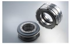
A GE-Thermodyn compressor - operated in the isomerization unit of the Tüpras Kirikkale refinery in Turkey - is safely sealed with EagleBurgmann dry gas seals type **DGS9/123**. Operating conditions: p = 12.6 bar (182 PSI); t = 38 °C ... 150 °C (181 °F ... 302 °F); n = 12,915 min<sup>-1</sup>; d1 = 103 mm (5.06"). Medium: mixture of hydrocarbons.
