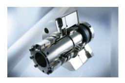
An EagleBurgmann **MFLWTS1/83** seals the shaft of a Leistritz screw pump in the de-asphalting unit of the ENI refinery in Sannazzaro de' Burgondi, Italy. Pump and metal bellows seals were started up in 2006. Operating conditions: p=1.87 bar (27 PSI); t=274 °C (525 °F); n=1,700 min<sup>-1</sup>; d1=75 mm (2.95"). Medium: asphaltene.
