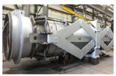
EagleBurgmann provided a large sized **universal spent catalyst standpipe expansion joint** for a refinery in Texas, USA. Operating conditions: p=...3.79 barg (55 PSIG); t=732 °C (1,350 °F); d=1,500 mm (59").
