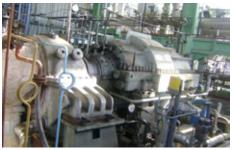
Bhel compressor in the delayed coker unit of the Panipat refinery run by the Indian Oil Corporation Ltd. The machine is equipped with EagleBurgmann **DGS20.1/200** tandem gas seals and a **diaphragm coupling**. Operating conditions: p=6 barg (87 PSIG); t=150 °C (302 °F); n=8,909 min<sup>-1</sup>; d1=180 mm (7.09"). Medium: flue gas.
