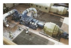
The two-stage screw compressor (Aerzen VR0825) used to compress coking oven gas in a coking plant is one of the biggest ever built. It is sealed with an EagleBurgmann type **HSH2/215**.
