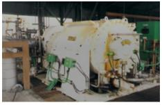
The hydro desulfurization unit of the refinery in Ciudad Madero, Tamaulipas, Mexico is equipped with a Mitsubishi compressor. It is reliably sealed by EagleBurgmann **SH6-D** dual mechanical seals. Operating conditions: p=3.4...5.6 bar (49 ... 81 PSI); t=20 °C ... 150 °C (68 °F ... 302 °F); n=5,460...8,190 min<sup>-1</sup>; d1=150 mm (5.91"). Medium: qas.
