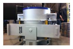
An Australian refinery has been fitted with a **cold** wall gimbal expansion joint (d = 1,067 mm (42")) and a **tied universal single expansion** joint (d = 889 mm (35")). Operating conditions: p = ... 4.14 bar (60 PSI); t = 750 °C (1,382 °F). Medium: flue gas.
