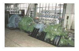
Coking oven gas compressor (Mannesmann Demag) at Wintershall AG, Lingen. Originally equipped with labyrinth seals, the turbine-driven single-shaft radial compressor has been converted to EagleBurgmann dual **DGS** seals and a buffer gas supply system. Operating conditions: p=5.6 barg (81 PSIG);  $n=12,800 \ min^{-1}$ ;  $d1=134.8 \ mm$  (5.3"). Medium: gas with  $H_2S$  content.
