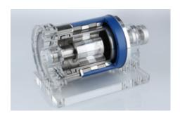
EagleBurgmann has designed a new high performance magnetic coupling type **NMB 22P-10R-65-ND2**. This is installed in a multistage vertical can pump of an ethylene cracker unit in a German refinery. p = ... 65 bar (943 PSI); t = -32 ... +40 °C (-26 °F ... +104 °F); n = 2,980 min<sup>-1</sup>; drive power: 315 kW direct start; design torque: >1,700 Nm. Media: hydrocarbons C2+C4.
