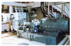
Hot steam has to be contained in a turbine at the Vapo Oy Pellet power station in Finland. An **Espey WKA400** carbon floating ring seal with steam and condensate leakage drain is used in this application. Operating conditions: p = 23 bar (344 PSI); t = 495 °C (923 °F); n = 8,200 min<sup>-1</sup>.
