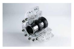
At the Olkiluoto (Block 3) nuclear power plant in Finland, a CVCS high-pressure feed pump which circulates radioactively contaminated reactor water must be absolutely reliable. An **SHFV-D4-/77-E1-Q** mechanical seal is used in this application. Operating conditions: p = 181 bar (2,625 PSI);  $t = 15 \dots 100$  °C (59 °F ... 212 °F); n = 2,980 min<sup>-1</sup>.
