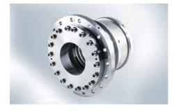
On a valve which closes isolation flaps in an emergency at the Olkiluoto (Block 3) power plant in Finland, an **Espey WKA600S** carbon ring floating seal with leakage drain is used to seal off the steam. Operating conditions: p = 11.6 bar (168 PSI); t = 311 °C (592 °F).
