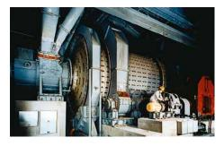
At the Dezhou Shandong Huaneng Power Development Co. Ltd. power plant in China, sealing air is used to contain hot exhaust air laden with coal dust in the neck of a coal mill. The ideal solution: An **Espey WD200/500**. Operating conditions: p = 1.08 bar (15.66 PSI); t = 110 °C (230 °F); n = 15.8 min<sup>-1</sup>.
