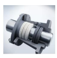
Insert more rings into the stuffing box making sure that each cut joint is at 90° to the previous ring joint. Rings should be added until the gland projects (for guidance) into stuffing box compartment by at least ¼ (for valves) or approx. ½ (for pumps) of the packing width "s". Press the rings home with the gland and tighten the nuts hand-tight. If there is a lantern ring, check that it is correctly positioned in relation to the inlet connection after the gland has been tightened.
