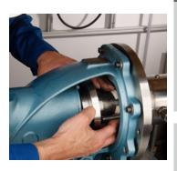
Using assembly shells, or the gland follower, each ring must be inserted separately into the stuffing box starting with the butted together cut ends. Pointed objects must never be used for this operation because there is a risk of damaging the shaft or deforming the packing material.
