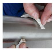
Die-pressed rings should be carefully twisted open in an axial and radial direction just far enough to enable them to be slipped over the shaft. Excessive bending of the rings can cause structural damage through kinking.
