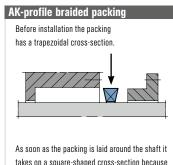
As soon as the packing is laid around the shaft i takes on a square-shaped cross-section becaus the material is squashed on the inside diameter and stretched on the outside diameter.
