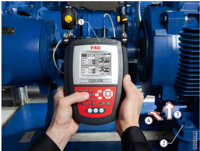
Figure 10 Finding the soft foot
