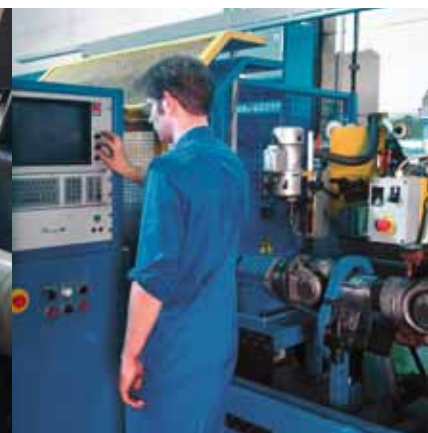
Computerised balancing technologies guarantee faultless performance of the Cardan shaft.
