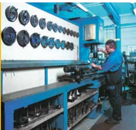
Pre-adjustment of the driveshaft on specially-designed straightening presses.
