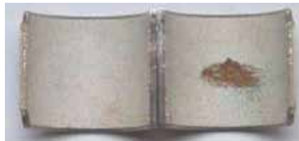
Fig. 34: Local damage caused by cavitation
