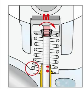
Cause: The spring was not inserted correctly during installation. The tilted spring had induced a lateral bending moment (M) on the valve stem.
