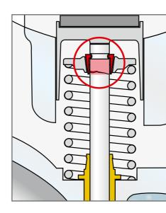
Cause: Old, worn valve cotters were used during replacement of the valves.
