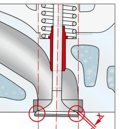
Cause: Non-centric remachining of the valve seat or guide.
