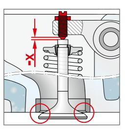
Cause: The valve clearance is set too tight or the maintenance intervals are exceeded.
