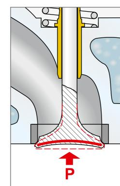
Cause: Significantly increased pressure and temperature loads occur in the combustion chamber as a result of abnormal combustion.
