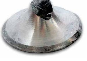
Result: The unilateral load causes the direction of the resulting bending load to change alternately from one side to another, causing fatigue fractures in the valve chamfer at the transition to the shaft or valve head.
