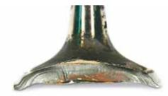
The valve head can no longer withstand the high thermal and mechanical loads and bends inwards. This results in the valve head being deformed into a so-called tulip shape and causes fractures in the area of the valve head
