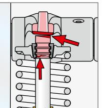
Cause: Forces are directed eccentrically from the rocker arm to the end face of the valve stem.
