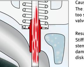
Cause: The guide diameter was dimensioned too small during replacement of the valve guides.
