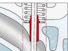
Cause: The valve guide clearance is too large due to excessive wear of the valve guides or due to excessive reaming during reconditioning.
