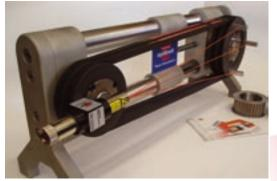
The Optibelt TT mini frequency tension tester is used to check the tension of drive belts by measuring their frequency of vibration. Due to its compact design, it offers universal
