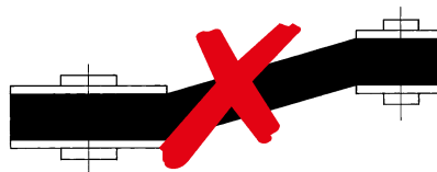
Axial misalignment of pulleys
