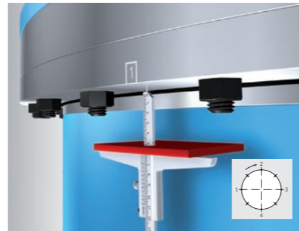
Figure 36: Basic setup for measuring the axial reduction with a depth gauge
