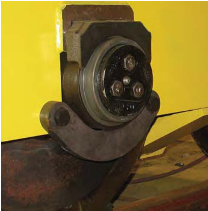
Fig. 8 Narrow adapter mounting on trolley safety bar
