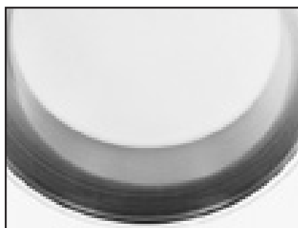
Fig. 38. Deflection, inaccurate machining or wear of bearing seats caused an irregular roller path on this tapered roller bearing outer ring.
