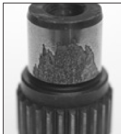
Fig. 36. High edge loads caused GSC spalling on the inner race of this drawn cup needle bearing.
