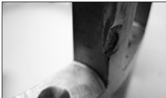
Fig. 51. Poor handling practices caused a deep dent on this spherical roller bearing cage bridge. This damage will result in a lack of proper roller rotation, possible roller skidding, increased temperatures and decreased life.
