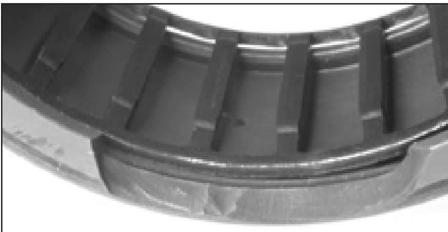
Fig. 45. A hardened driver caused a broken rib on this needle roller bearing.
