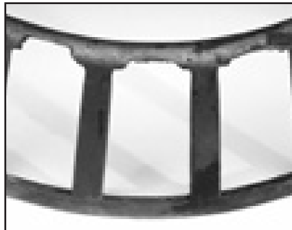
Fig. 35. Heavy wear in the small end of the cage pockets is typical of excessive endplay.
