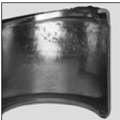
Fig. 73. High loads and extreme misalignment caused roll out of this needle roller bearing outer ring.
