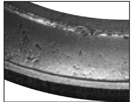
Fig. 30. High load and low speed conditions caused severe peeling and wear on this needle thrust race.
