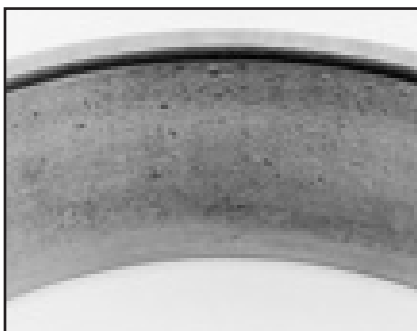
Fig. 10. Debris from other fatigued parts, inadequate sealing or poor maintenance caused bruising on this tapered roller bearing race.
