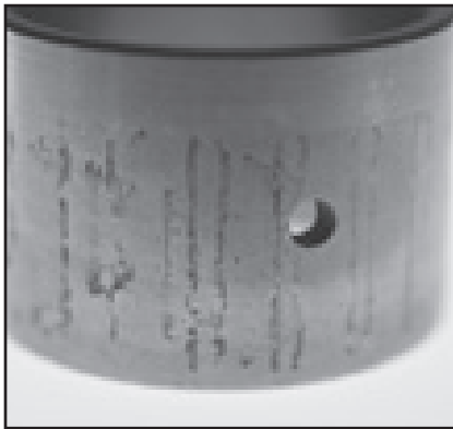
Fig. 12. This cylindrical bearing inner ring has etching and corrosion.
