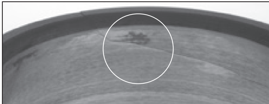
Fig. 58. This ball bearing inner ring fracture is a result of being installed on top of a metal contaminant or raised metal nick.
