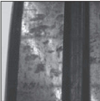
Fig. 52. A worn-out housing caused this bearing to lose fit and fret (move) during service. As a result, metal tearing and wear on this spherical outer ring occurred.
