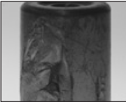
Fig. 28. Overloading on this cylindrical roller bearing caused roller surfaces to fracture.
