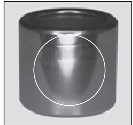
Fig. 54. Inaccurate machining caused a pinch point on this needle roller bearing and grooved the outer ring outside diameter.
