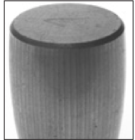
Fig. 71. Welding on a machine, while the bearings were rotating, caused electric arc fluting on this spherical roller bearing.
