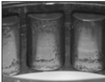
Fig. 26. High loads resulted in fatigue spalling on this cylindrical roller bearing.
