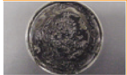
Fig. 81. This petri dish above contains heavily oxidized grease, which purged from an overfilled bearing. Grease undergoing heavy oxidation often has a very distinguishable black color and burned odor. In addition, it gets stiffer in consistency.
