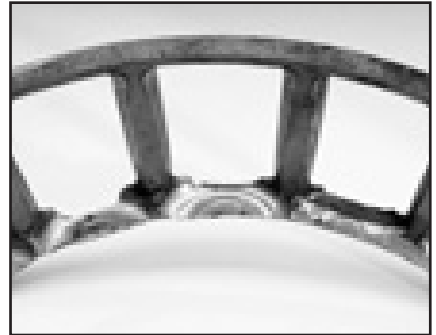
Fig. 34. Cage pocket damage from excessive roller movement.
