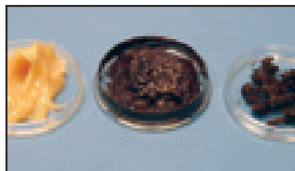
Fig. 89. The above photo shows the same grease at three stages from left to right. 1) new grease, 2) heavily oxidized grease, and 3) worn-out (failed) grease where the thickener and additives have decomposed and the oil has broken down.
