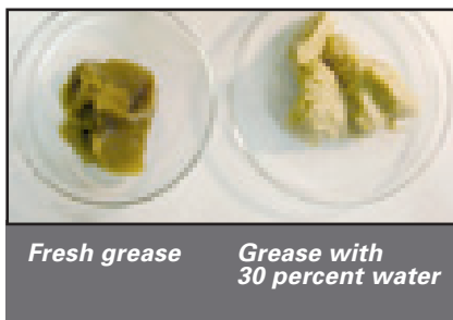
Fig. 91. The effect of water on grease is depicted here.
