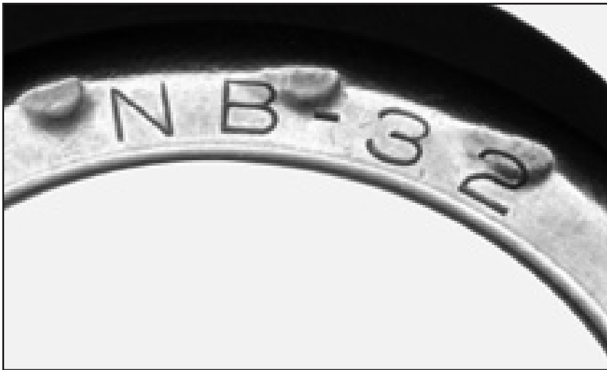
Fig. 46. A hardened punch caused indents during assembly.
