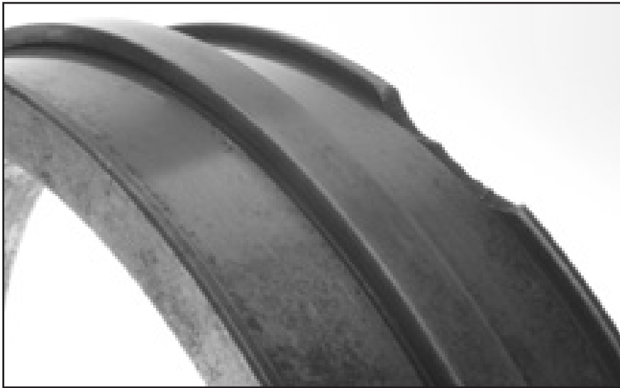
Fig. 43. This spherical roller bearing inner race depicts a fractured small rib caused by the use of improper installation tools.
