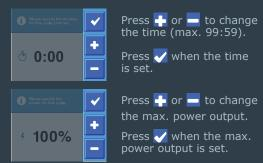
When using smaller yoke sizes on a SURE**THERM PRO** heater, make sure to reduce the maximum power output. See **page 13** for an overview of the advised max. power output per yoke size.
