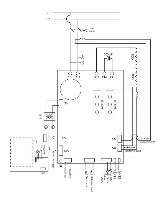
Electrical drawing SURETHERM PRO  $6 \times$
