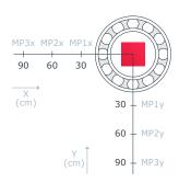
conforming to local regulations regarding the maximum time exposure to magnetic fields. Different configurations may give different values. It is impossible to provide values for all combinations as the variety of bearing types in combination with the different yokes is large.
