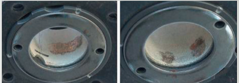
Fig. 37: P2 plain bearing, grooves in the sliding surface
