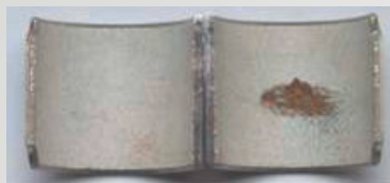
Fig. 35: Local damage caused by cavitation
